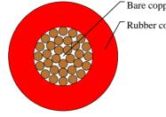
Bare copper conductor Rubber compound insulation
